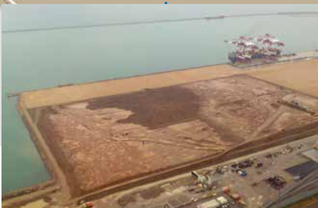
MOVEMENT OF PRE-LOADED MATERIALS (ACTION 6) PRAT TERMINAL
