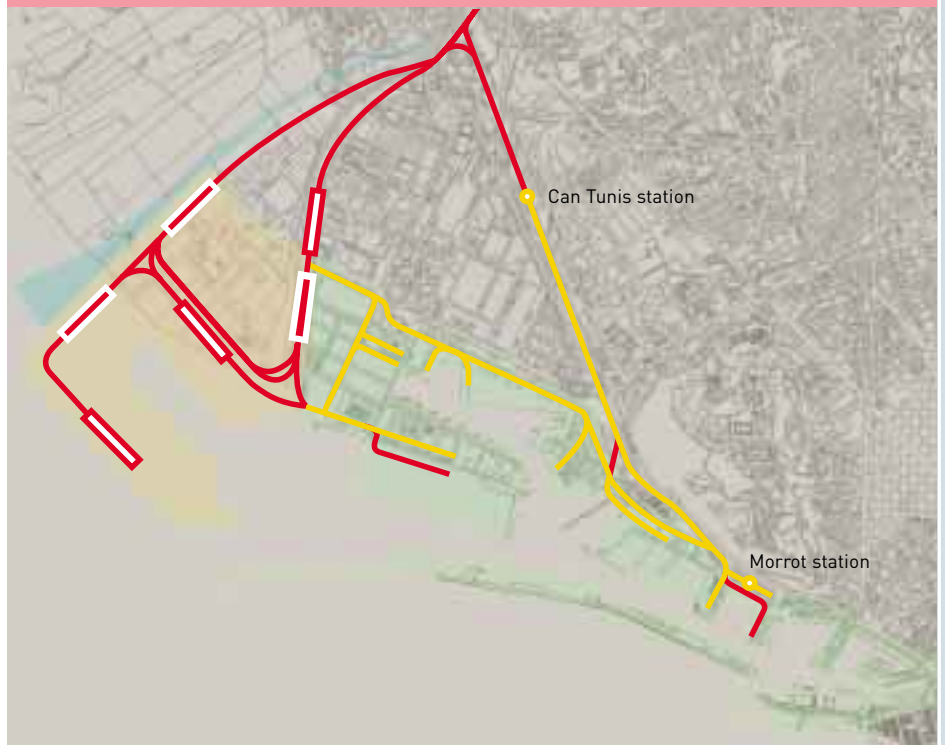
—○— Current Iberian gauge rail connections Loading / unloading terminals — Future mixed gauge rail connections Receiving / sending terminals
