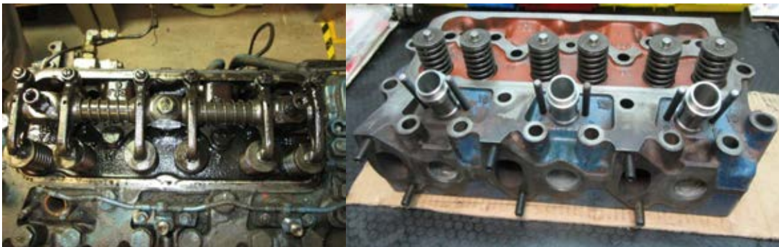
Figure 18: Comparison between the original engine and after cleaning process
