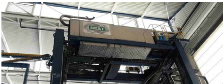
Figure 41. PEMS installed on the top of the Straddle Carrier
