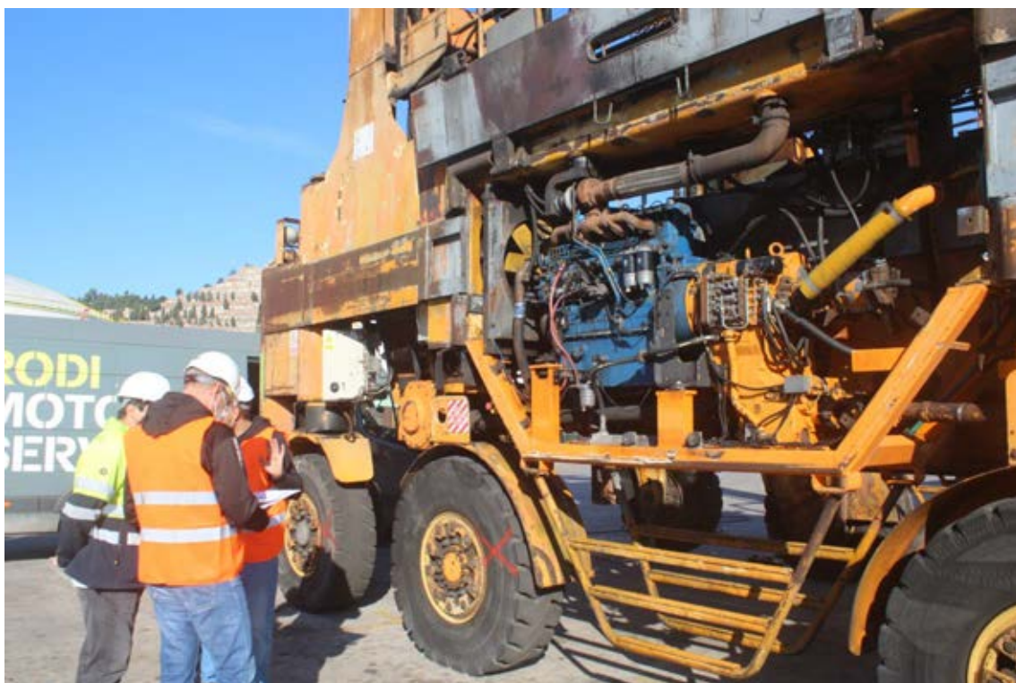
Figure 80. Engine installation at the APMT straddle carrier.
