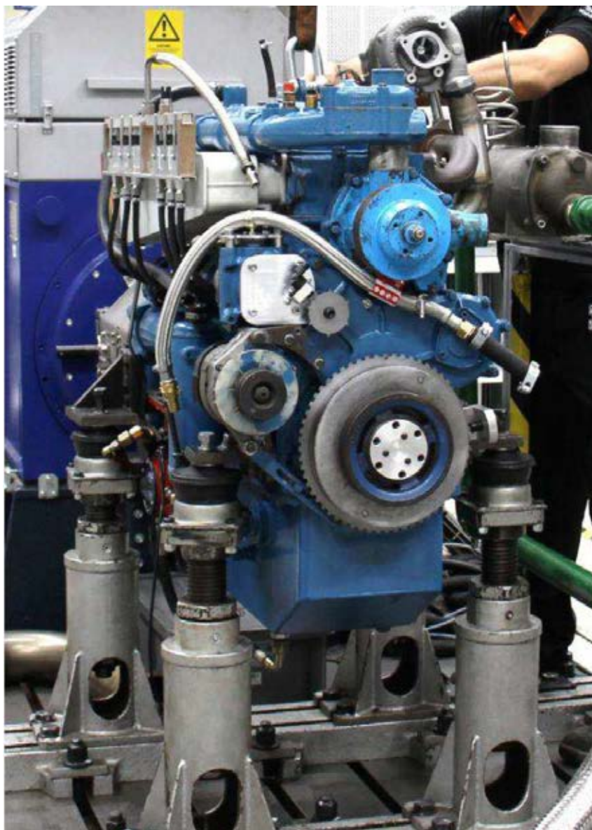
Figure 52. First converted engine installed in test bench
