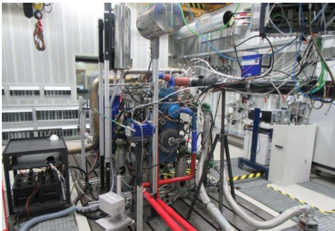
Figure 53. Engine installation in the test bench with instrumentation.
