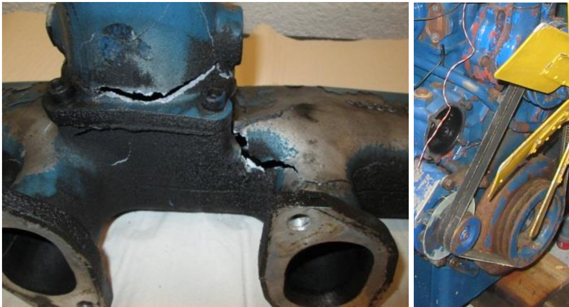
Figure 15: Deterioration of the original intake manifold and V-belt.
