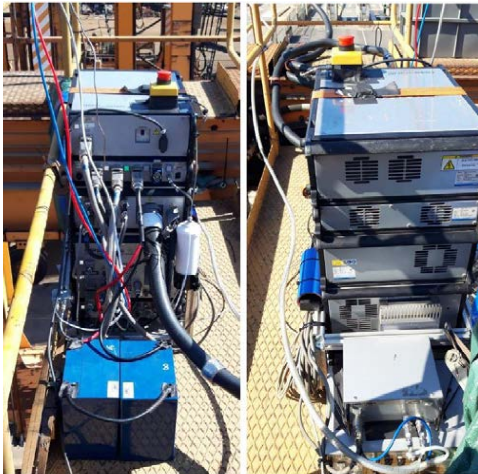
Figure 64. PEMS installed on top of the straddle carrier, front and back side views
