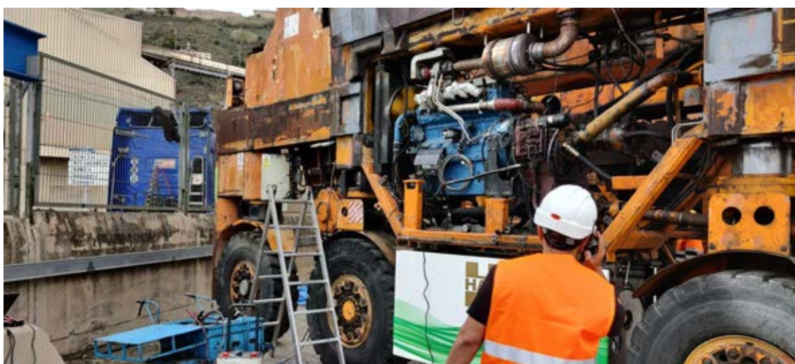
Figure 81. Natural gas engine calibration and emissions measurements (PEMS)
