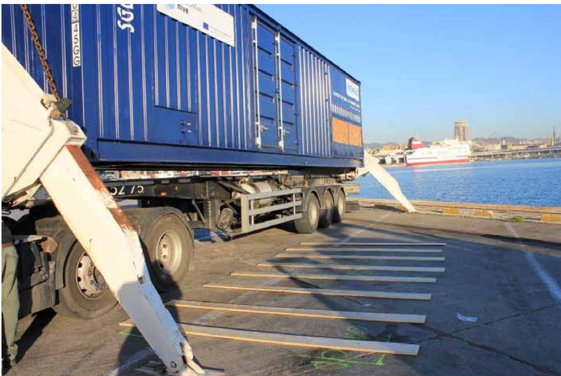
Figura 15. Placing wooden planks to properly support the generator engine.
