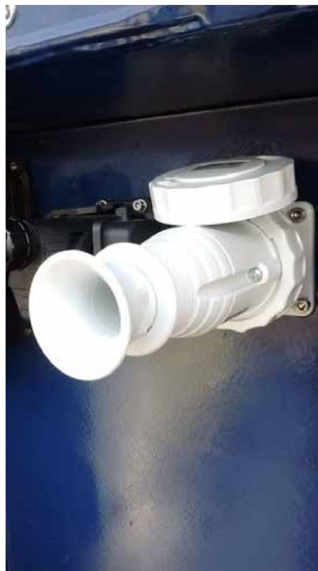
Figure 19. Pratika 82977 connector, to connect the 24 V socket to the motor container.
