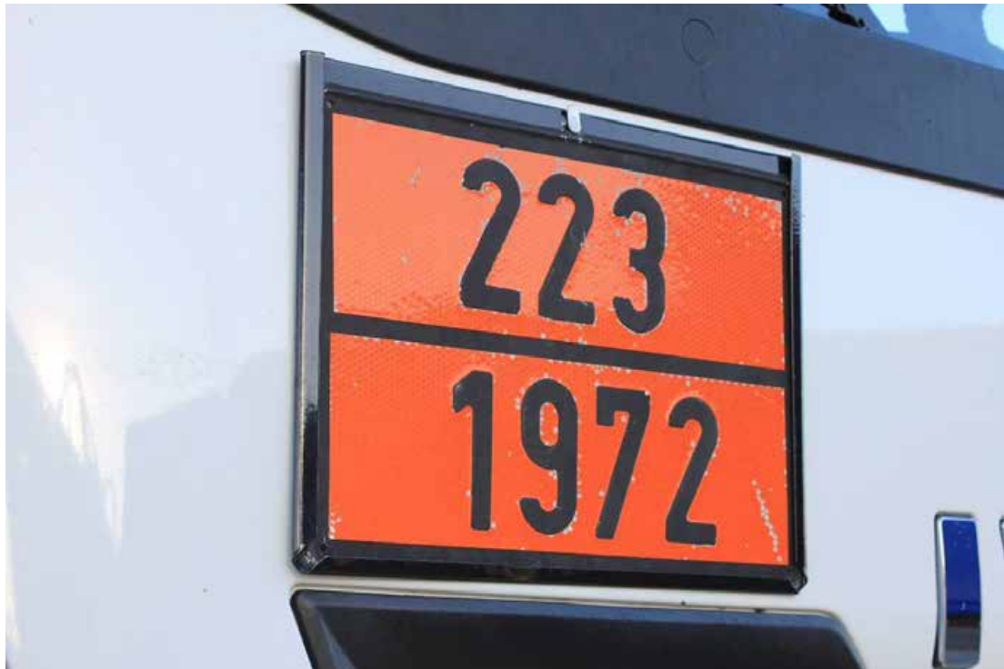
Figura 115. Dangerous goods transport registration (ADR). The number 223 is the hazard number (refrigerated liquefied gas, flammable) and the number 1972 represents LNG.
