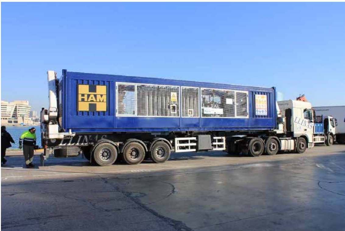
Figura 17. Loading the container of the LNG tanks on the sidelifter and positioning it at the agreed site.
