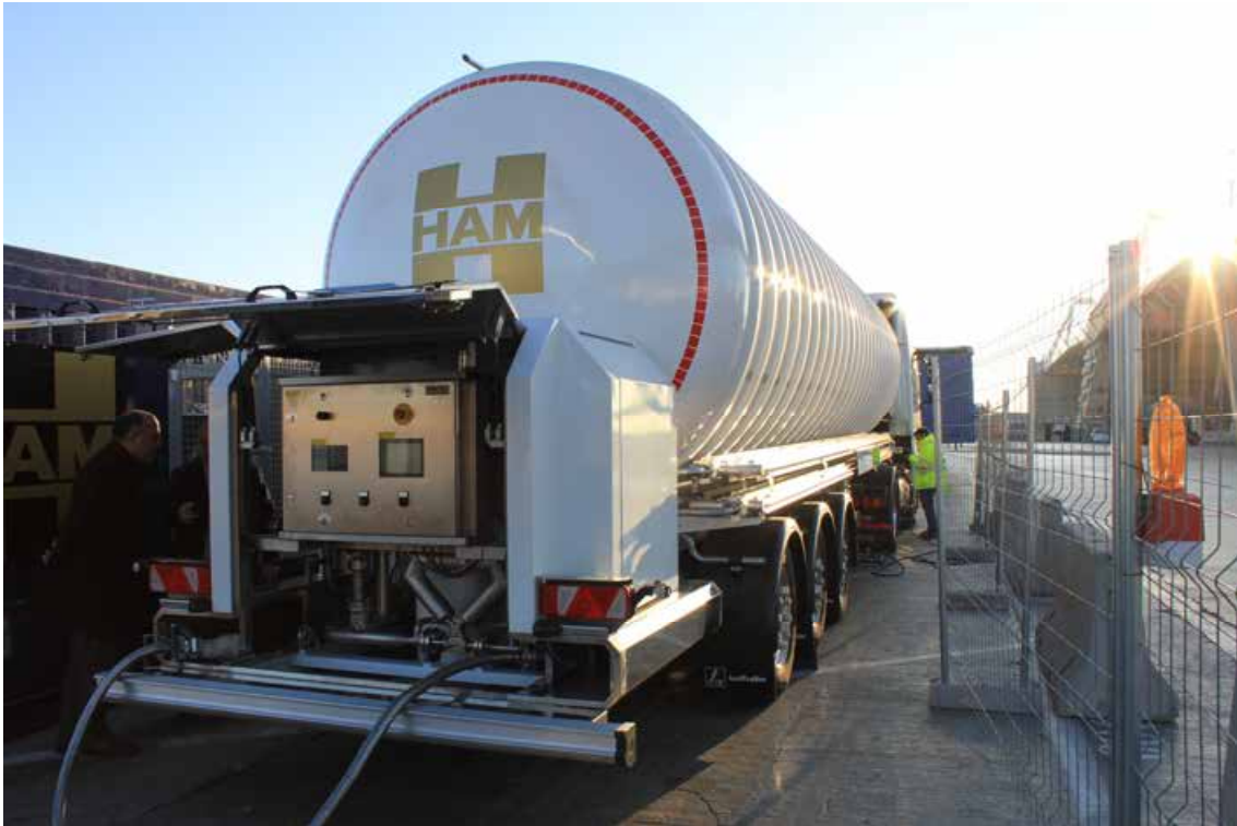
Figure 17. Mobile service station. Detail of the dispenser and control panels.
