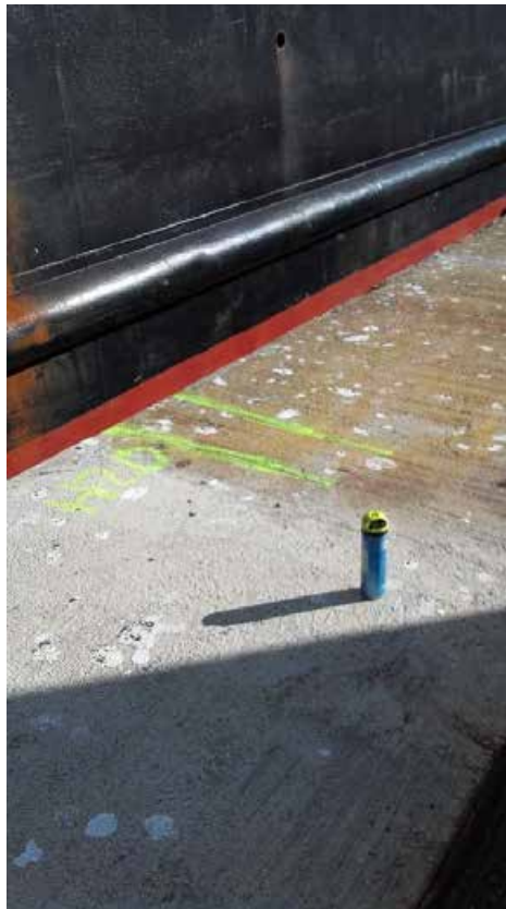
Figura 11. Marking the position of the engine cooling pipes.
