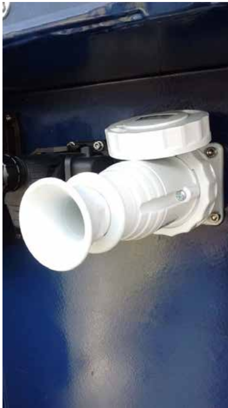
Figura 42. Pratika 82977 connector, to connect the 24v socket to the engine container.
