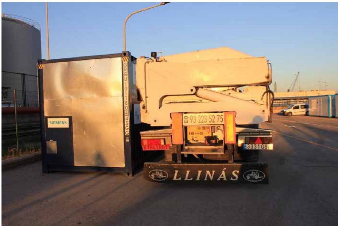
Figura 13. Loading the container of the Guascor-Siemens generator engine located at the Enagás plant with the truck with sidelifter.
