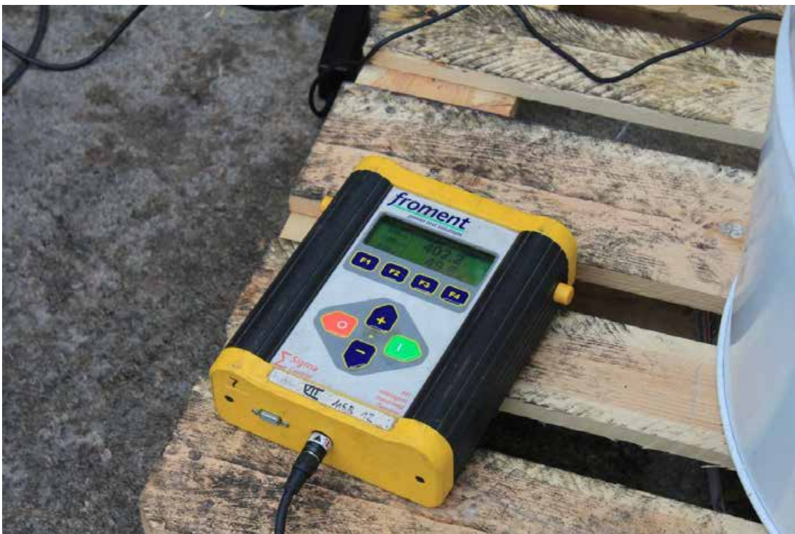
Figura 148. Voltage and frequency measurement equipment.
