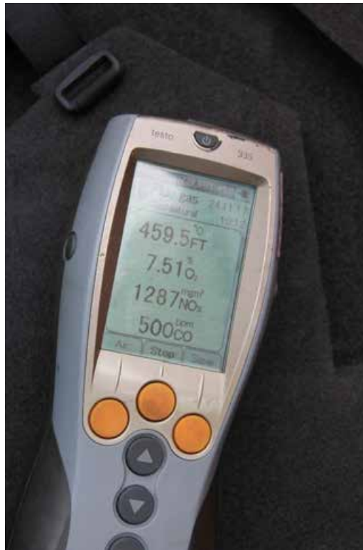
Figura 151. Gas probe for measuring exhaust emissions. Exhaust temperature, % O 2 , mg/m 3 NO x or ppm of CO.
