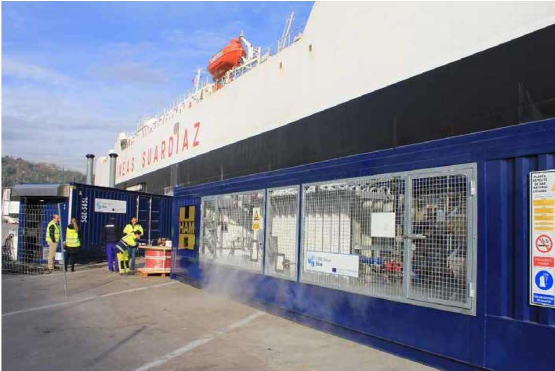
Figure 11. Pilot of 24 November 2017. All equipment. It is possible to make out the condensation of the ambient humidity due to the cold of the LNG plant.
