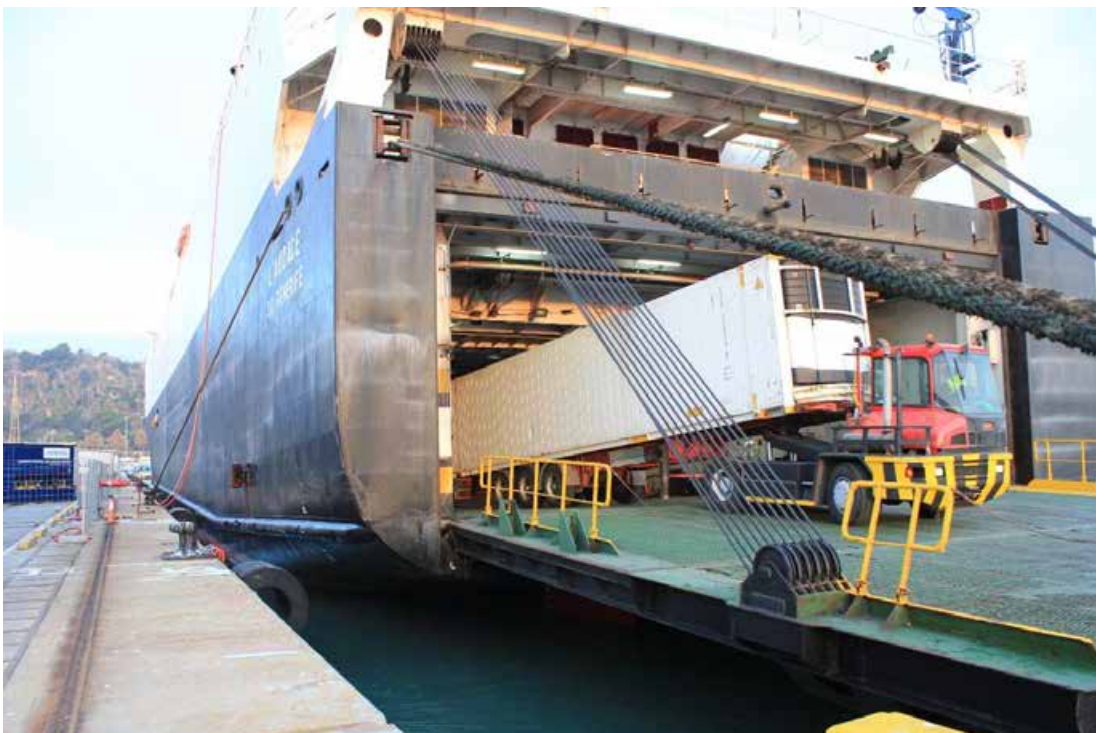
Figura 161. Pilot of 8 December. Ship in operation. Charging a reffer (refrigerated container, with high energy consumption on the ship).
