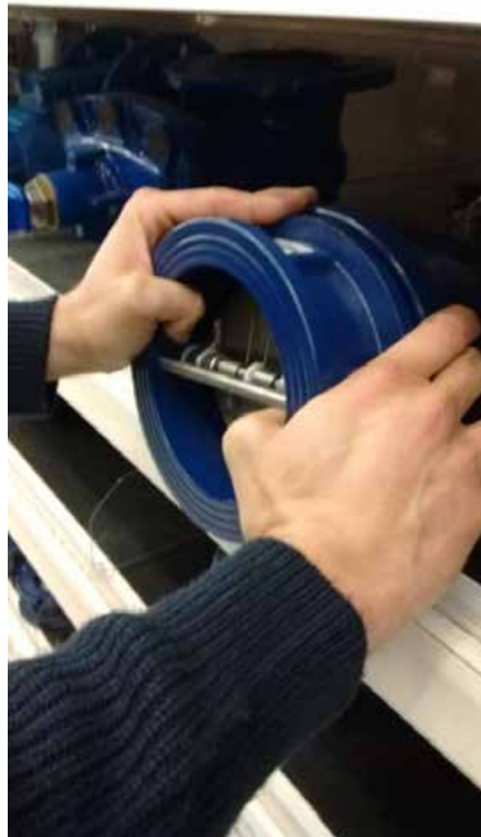
Figura 65. Non-return valve, similar to the one that was finally installed at the end of the seawater inlet pipe.
