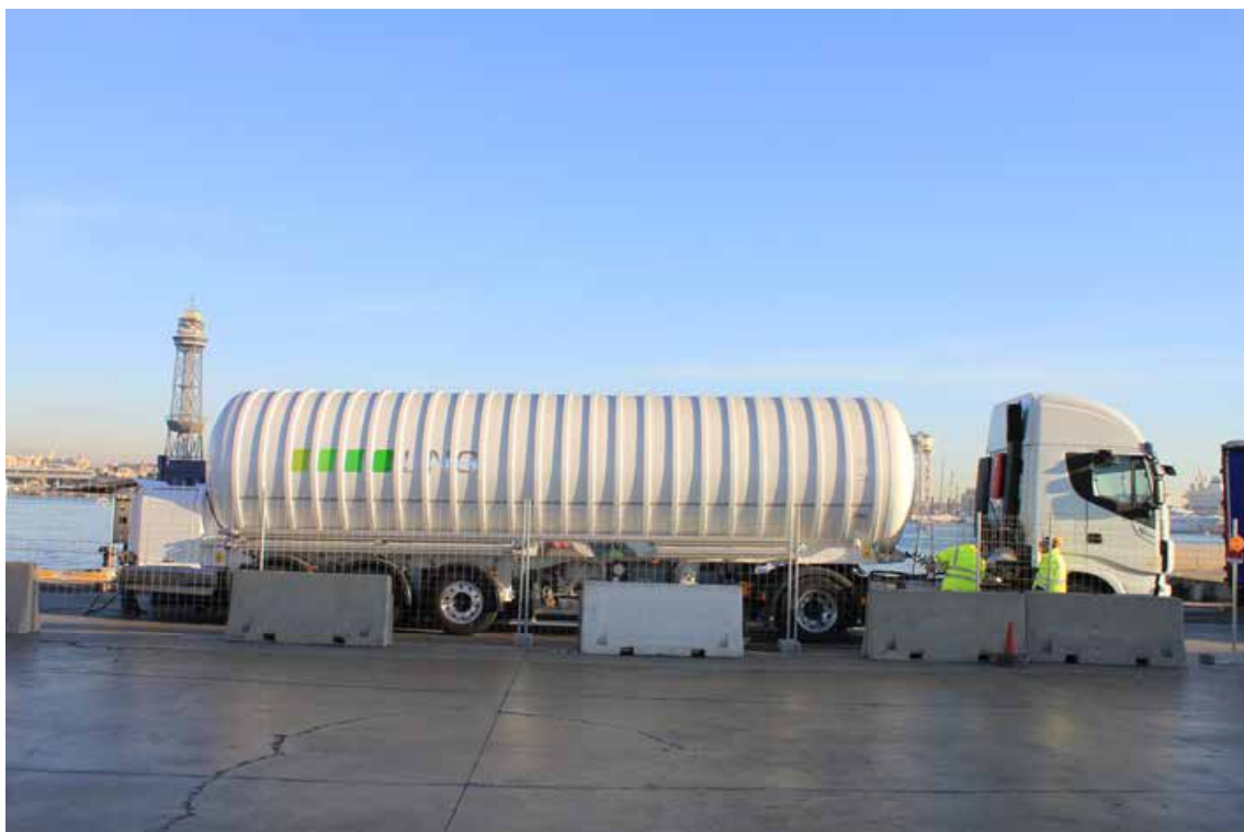
Figure 16. Mobile service station.
