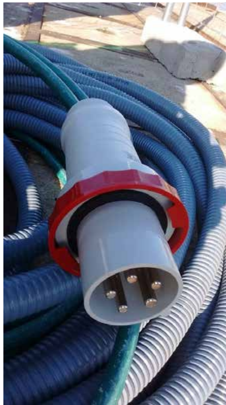
Figure 17. Pratika 81683 connector, to connect the 400 V socket to the motor container.
