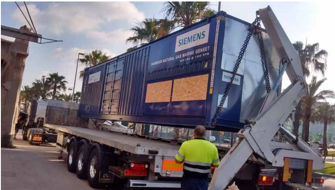
Figure 5: Lifting the engine container with a Sidelifter (hitch on each side of the container).
