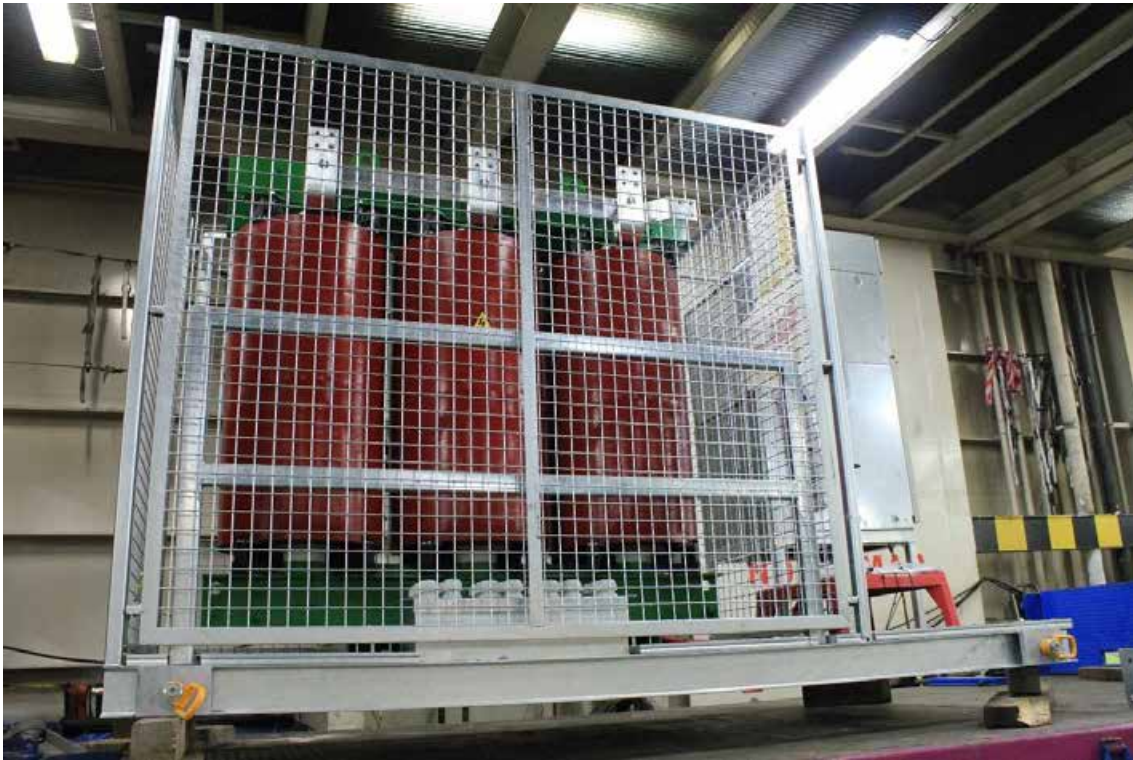
Figura 99. Ship's transformer (before installation).
