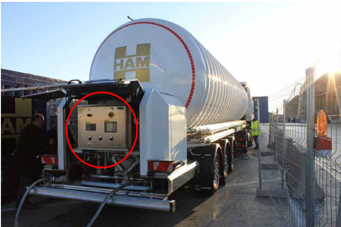
Figura 114. LNG tanker with the tractor facing outwards. In red, measurement system of the supplied LNG and control of the tanker valves.
