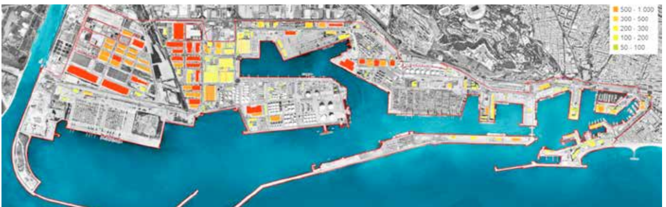
Map of the photovoltaic potential on roofs in the port area (in kW peak).
