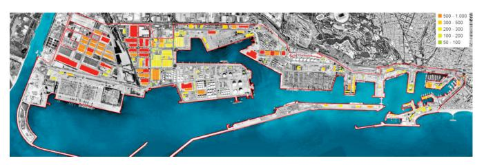
Map of the photovoltaic potential on roofs in the port area (in kW peak).
