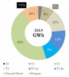
**Figure 4.4:** 2015 POLA cargo handling equipment energy consumption, by engine type & US EPA non-road diesel engine tier
