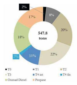
**Figure 4.5:** 2015 POLA cargo handling equipment NO<sub>x</sub> emissions, by engine type & US EPA non-road diesel engine tier
