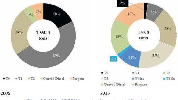
**Figure 4.8:** 2005 vs 2015 POLA cargo handling equipment NO<sub>x</sub> emissions, by engine type & US EPA non-road diesel engine tier, tons
